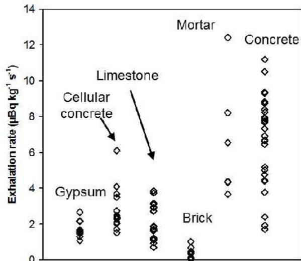
Figure 1 Overview of the radon exhalation from building materials in the Netherlands.
